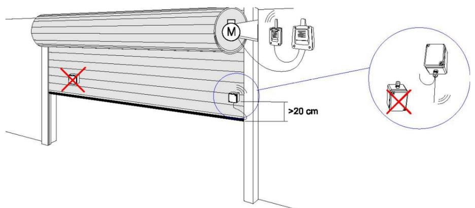
Installation on horizontal sectional powered door or gate with control panel and PSSW/RX
