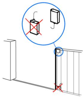
Do not fit the equipment at ground level.
