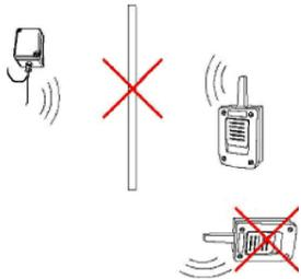
The transmitter and receiver antennae must be parallel to each other for optimum signal reception
