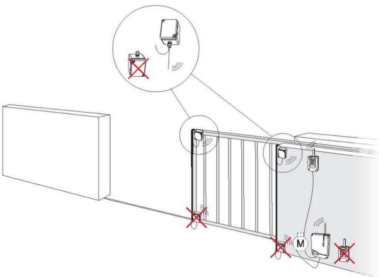
Installation on roller powered door or gate with control panel and PSSW/RX.
